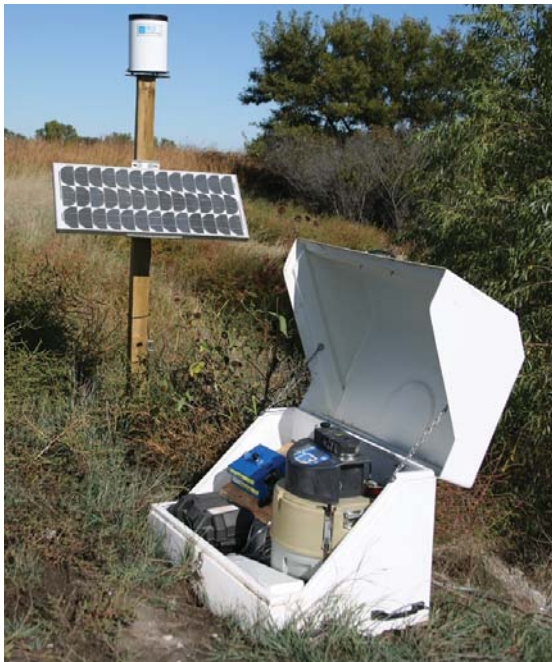
The 2105 system shown above interfaces a rain gauge, flow meters, automatic sampling, and a multi-parameter sonde.
