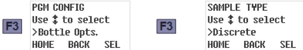
15. Press F3 to accept that setting and view the sequential BOTTLE CONFIGURATION. This is factory set to match the carousel you purchased, so you shouldn't need to change it. If you do, use the Up or Down key to scroll to the desired configuration:
