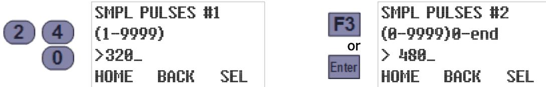
The digit keys can then be used to change the number of pulses the program would wait between initiating its first and second samples. Pressing the SEL [F3] or Enter key would again save the displayed value and display the next. And so on until pressing the SEL [F3] or Enter key while Sample Pulses #24 is displayed restores the Program Configuration menu scrolled to its next group (Bottle Options):
