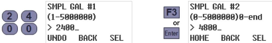
The digit keys can then be used to change the number of gallons the program would measure between initiating its first and second samples. Pressing the SEL [F3] or Enter key would again save the displayed value and display the next. And so on until pressing the SEL [F3] or Enter key while Sample Gallons #24 is displayed restores the Program Configuration menu scrolled to its next group (Bottle Options):
