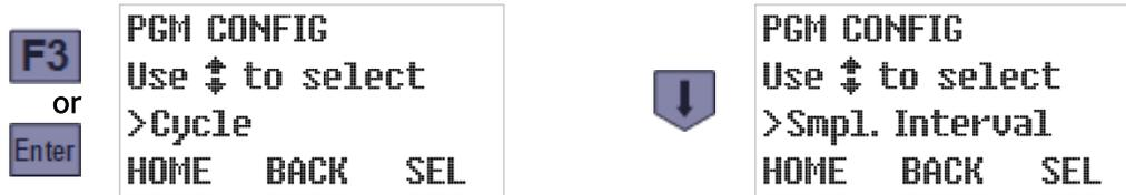
Press the SEL [F3] or Enter key to display the currently-configured interval type, then use the Down or Up key to scroll to the desired new setting. With that value displayed, press the SEL [F3] or Enter key to display the first parameter for that interval type:
