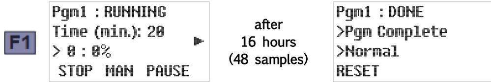
21. You should then replace the sample carousel with one containing empty bottles and press F1 to reset the program. Then repeat Step 20 twenty minutes before you want to start the next day's sampling.
