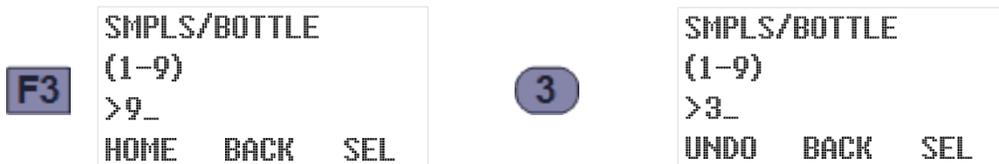
18. Press F3 to accept that setting and view the the bottle indexing option the program is currently set to use. If necessary, use the Up or Down key to scroll to the desired option. In this example, we would select the After Bottle setting so the program would discharge three samples to each bottle and then rotate to the next:
