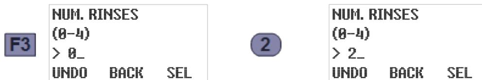
6. Press F3 to accept that setting. If it is not zero, the rinse cycle PRESSURE TIME will then be displayed. Then type the number of seconds each rinse should pressurize the sample chamber (e.g., 8):
