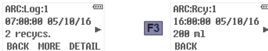
where the screen shown to the left indicates two of our example program run's sample cycles needed more than one vacuum phase to fill the sample chamber. The screen on the right indicates the first such sample cycle was initiated at about 4:00 PM.
