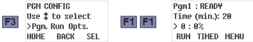
20. Twenty minutes before the first sample is to be drawn, press F1 to start the sampling program. Barring unforeseen problems, that program would then run for 16 hours and stop:
