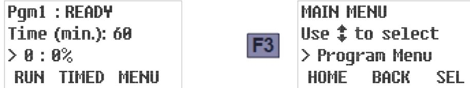
If that password has a non-zero value, the Password entry screen will appear instead. Like many other menu screens, it assigns the HOME, BACK and SEL[ect] functions to the F1, F2 and F3 keys:
