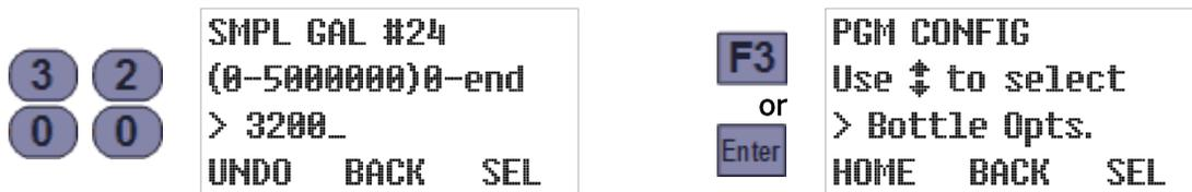
However, you do not need to set all 24 intervals—setting any one of them to 0 configures the program to use the value of the preceding parameter for all subsequent intervals. For example, setting Sample Gallons #5 to 4000 and Sample Gallons #6 to 0 would have the same effect as setting Sample Gallons #6 through #24 all to 4000 (the value of Sample Gallons #5):
