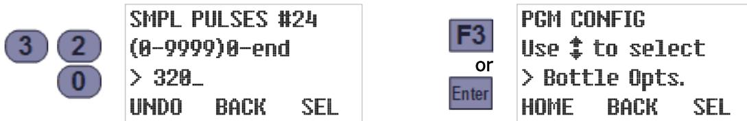
However, you do not need to set all 24 intervals—setting any one of them to 0 configures the program to use the value of the preceding parameter for all subsequent intervals. For example, setting Sample Pulses #5 to 400 and Sample Pulses #6 to 0 would have the same effect as setting Sample Pulses #6 through #24 all to 400 (the value of Sample Pulses #5):
