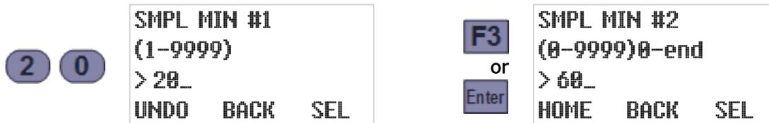
The digit keys can then be used to change the number of minutes the program would wait between initiating its first and second samples. Pressing the SEL [F3] or Enter key would again save the displayed value and display the next. And so on until pressing the SEL [F3] or Enter key while Sample Minutes #24 is displayed restores the Program Configuration menu scrolled to its next group (Bottle Options).
