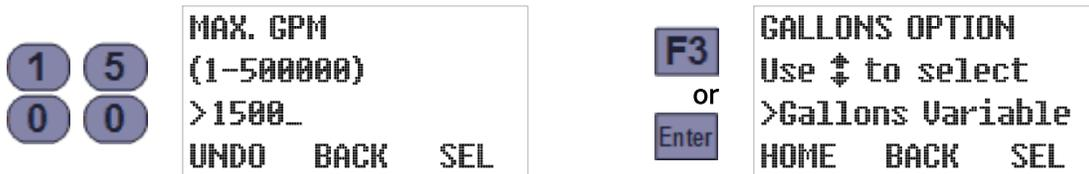
The above example assumes you are using a flow transmitter whose signal varies from 0 Vdc at no flow up to 10 Vdc at 1500 gallons per minute. A 1.0 Vdc signal would then indicate the flow was 150 gpm, so the controller would then calculate the instantaneous flow by multiplying 150 by the input signal in volts.
