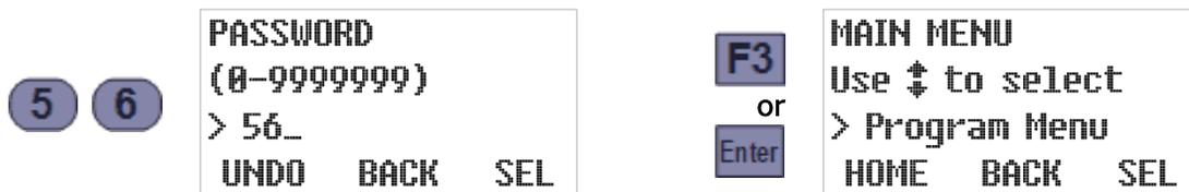
Typing the first digit changes the F1 prompt to UNDO—pressing that key would then clear any digits you had typed so far and restore the initial Password screen. In contrast, pressing BACK [F2] or the Back key will clear only the last typed digit.
