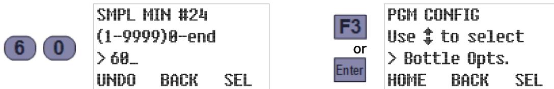
However, you do not need to set all 24 intervals—setting any one of them to 0 configures the program to use the value of the preceding parameter for all subsequent intervals. For example, setting Sample Minutes #5 to 120 and Sample Minutes #6 to 0 would have the same effect as setting Sample Minutes #6 through #24 all to 120 (the value of Sample Minutes #5):
