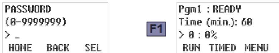
To access the Main Menu, use the numeric keys to type the correct password, then press SEL [F3] or the Enter key. If the password was 56, for example:
