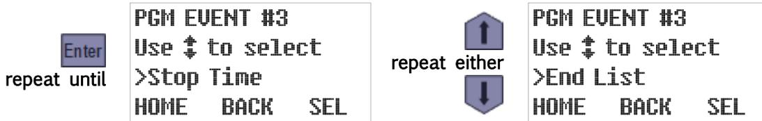
3. Finally, press SEL [F3] or the Enter key to delete this and any higher-numbered events:
