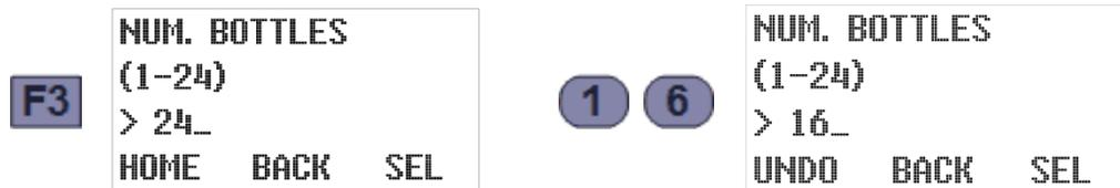
17. Press F3 to accept that setting and view the number of samples each container is currently set to receive. Then type the number that should be discharged to each bottle (e.g., 3):
