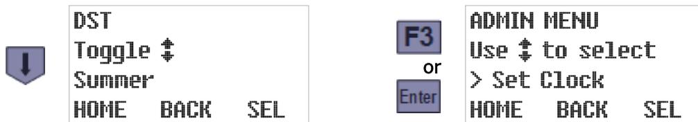
3. To adjust the date and time settings, press the SEL [F3] or Enter key. Otherwise, scroll to another Administration Menu option or press the HOME [F1] key to restore the Main Menu. The current date setting is displayed first. If it is correct, or after you have corrected it, press the Enter key to save the displayed date and access the current time setting:
