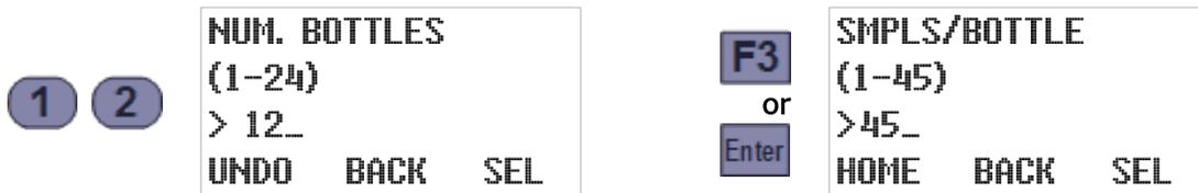
The numeric keys can then be used to change that number, and pressing the SEL [F3] or Enter key will again save the displayed value and display the currently bottle indexing setting:
