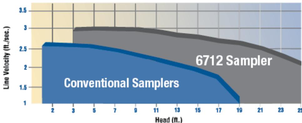
The 6712 pump is not as affected by varying head heights as other samplers. From one sample to the next, the 6712 pump eliminates variability in sample content due to inconsistent sample velocities.
