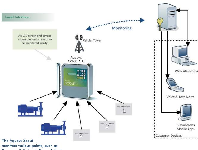
Pump run/fail, Level, Power Fail, etc.
