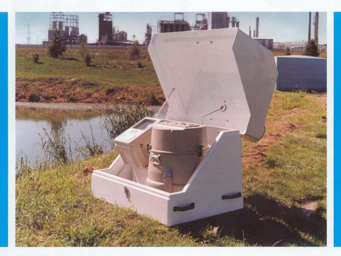
Many water monitoring applications require a system to monitor rainfall, measure flow, and take automatic samples at remote locations. Most sites are unattended and unprotected leaving all components exposed to the elements.
